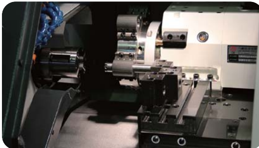
六刀位刀塔將提升高效率 Turret increases turning efficiency
